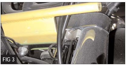
**NOTE:** Put the clutch cable over the brackets before installing the side brackets.
