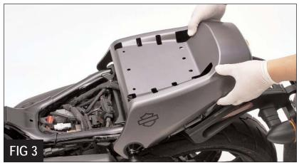
5. To install your saddle, slide the front tab on the saddle under the tab at the rear of the gas tank, then align the rear of the saddle with the latch pin you just installed. Push down until you hear it click *(Figures 7).*
