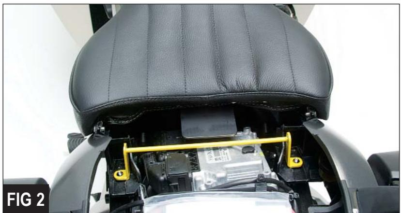
4. **Front Saddle:** Slide the front tongue into the bracket at the base of the gas tank.
