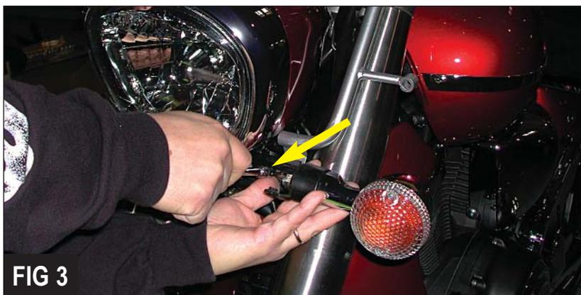
**NOTE:** These bolts can prove to be a bit difficult to remove. Make sure you use a good Allen tip to prevent bolt from stripping.
