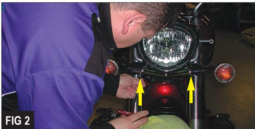
4. Remove the bolts from the turn signal using a 5mm Allen key (*Figure 3*).
