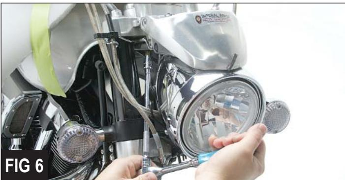
11. Reinstall the light housing and gauge unit using the stock bolts. Use Loctite®.
