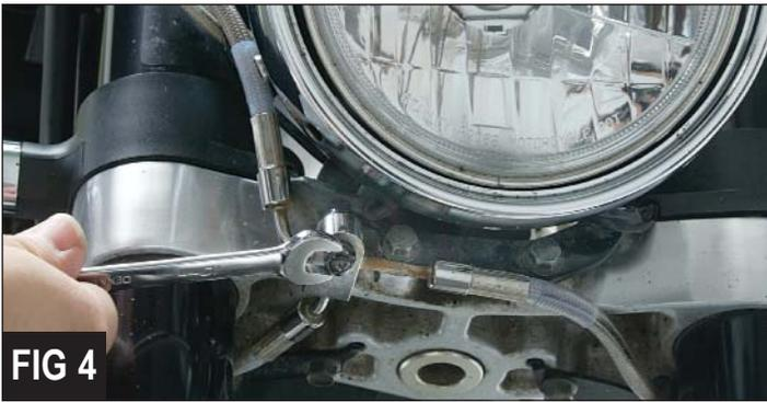
**NOTE:** These bolts are hard to reach. Using an open wrench will make it easier.
