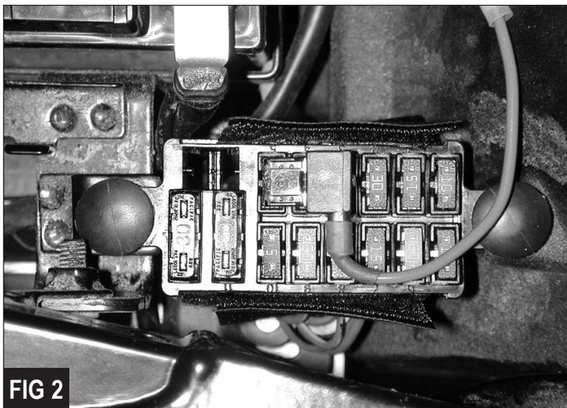
8. With the adapter in place, the fusebox cover will not snap back into place. Instead, we will be attaching the cover with the included velcro strips. Attach two of the 1" x 2" female pieces on the sides of the fusebox cover and two on the sides of the fusebox itself. Now set the cover in place and hold it there using the two 2" x 2" male pieces to secure the cover to the fusebox. There is an illustration located at Figure 4... it will make more sense when you look at it.
