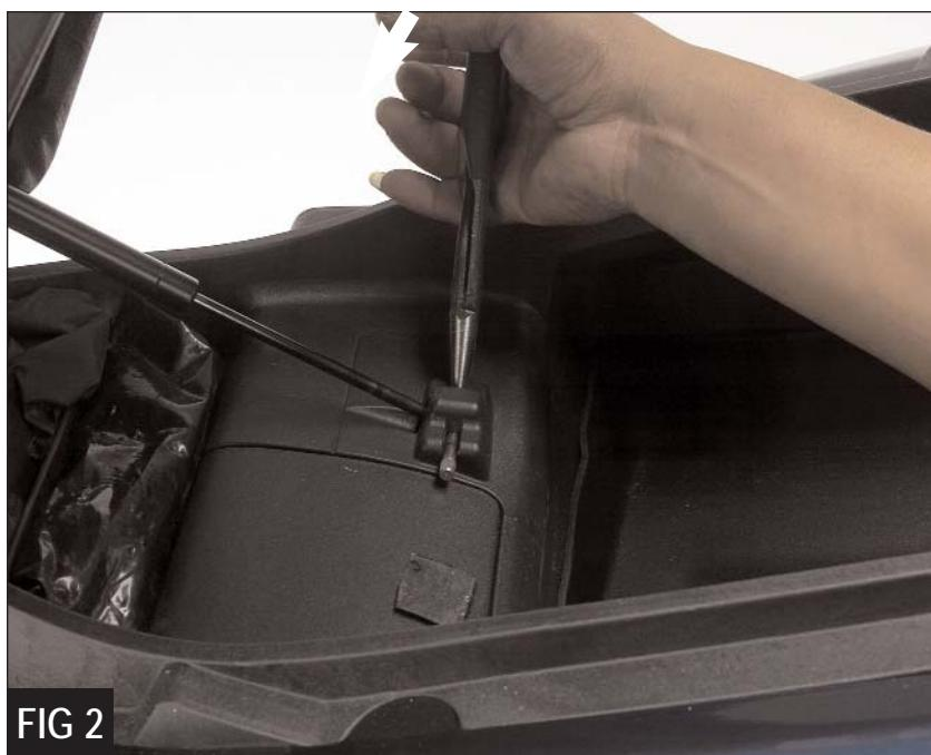
5. To latch the seat, firmly press the seat down over the latch to lock into place.
