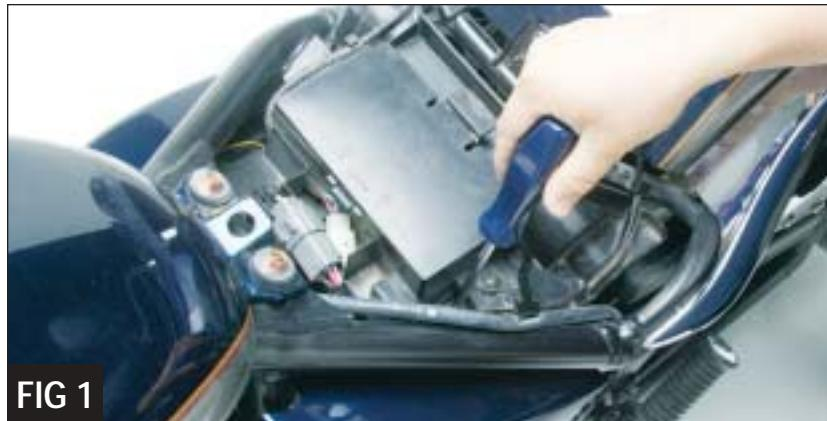
2. For safety considerations, we recommend disconnecting the positive lead from the battery terminal while working on your motorcycle.
