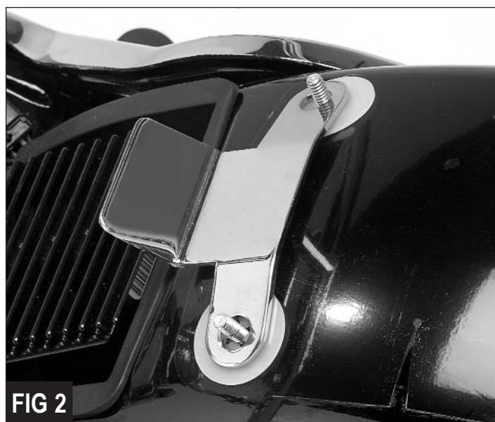
5. Install the supplied latch pin as shown in *Figure 5*, using the supplied 1/4-20 x 3/4" flat head socket cap screws, using a 5/32" Allen wrench. Tighten to 8 ft lbs.
