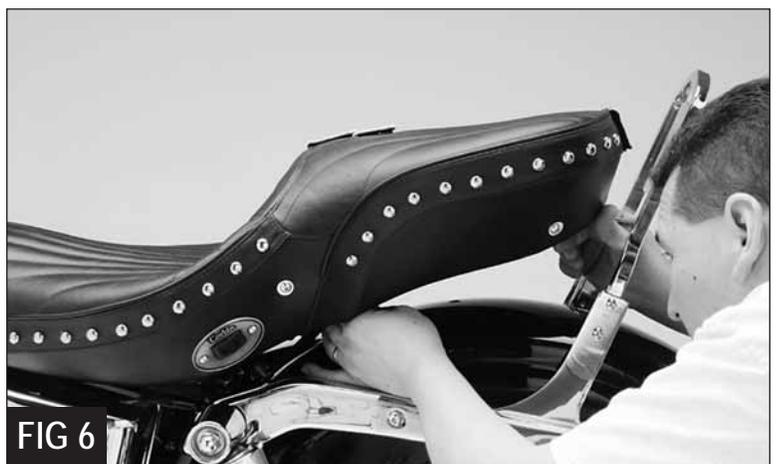
e) Plug the wiring pigtail on the Corbin saddle into the wiring harness you just installed. Flip the switch on the saddle. If the switch illuminates, the saddle heater is working.
