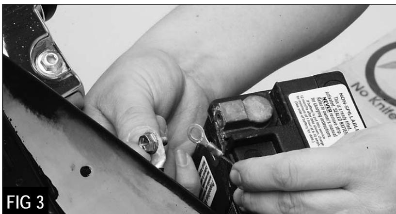
8. Install the black wire onto the negative terminal of your battery under the original ground as shown in *Figure 3*. Tighten securely and slide your battery back into place. You may now reinstall the battery cover.
